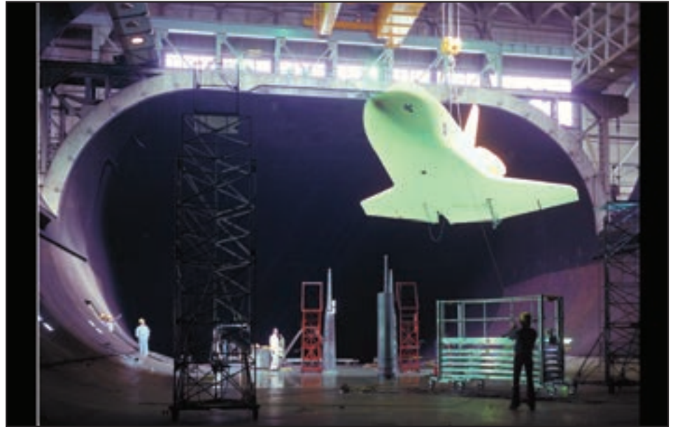
In 1975, a scale model of the space shuttle orbiter is installed into the 40 by 80-foot wind tunnel at the NFAC for subsonic aerodynamic testing of what the vehicle would experience during the latter stages of re-entry. (NASA photo by Lee Jones)
