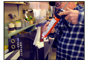
An AEDC craftsman applies adhesive to bond foam seal to a C1 spacer.
