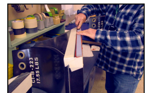
Installing foam seal to a C1 spacer.
