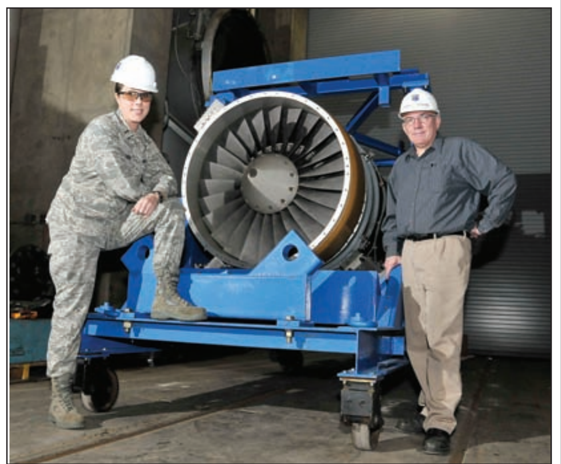
The Rolls-Royce AE3007H growth engine, the power plant for the RQ-4 Global Hawk unmanned aircraft system (UAS), is now being tested at AEDC under the eye of 717th Test Squadron Project Manager 2nd Lt. Jamie Gurganus and ATA Project Engineer Andrew Jackson. The engine has upgraded turbine hardware and an improved combustor that, if validated by this project, will enable the engine to have greater service life. (U.S. Air Force photo by Rick Goodfriend)
