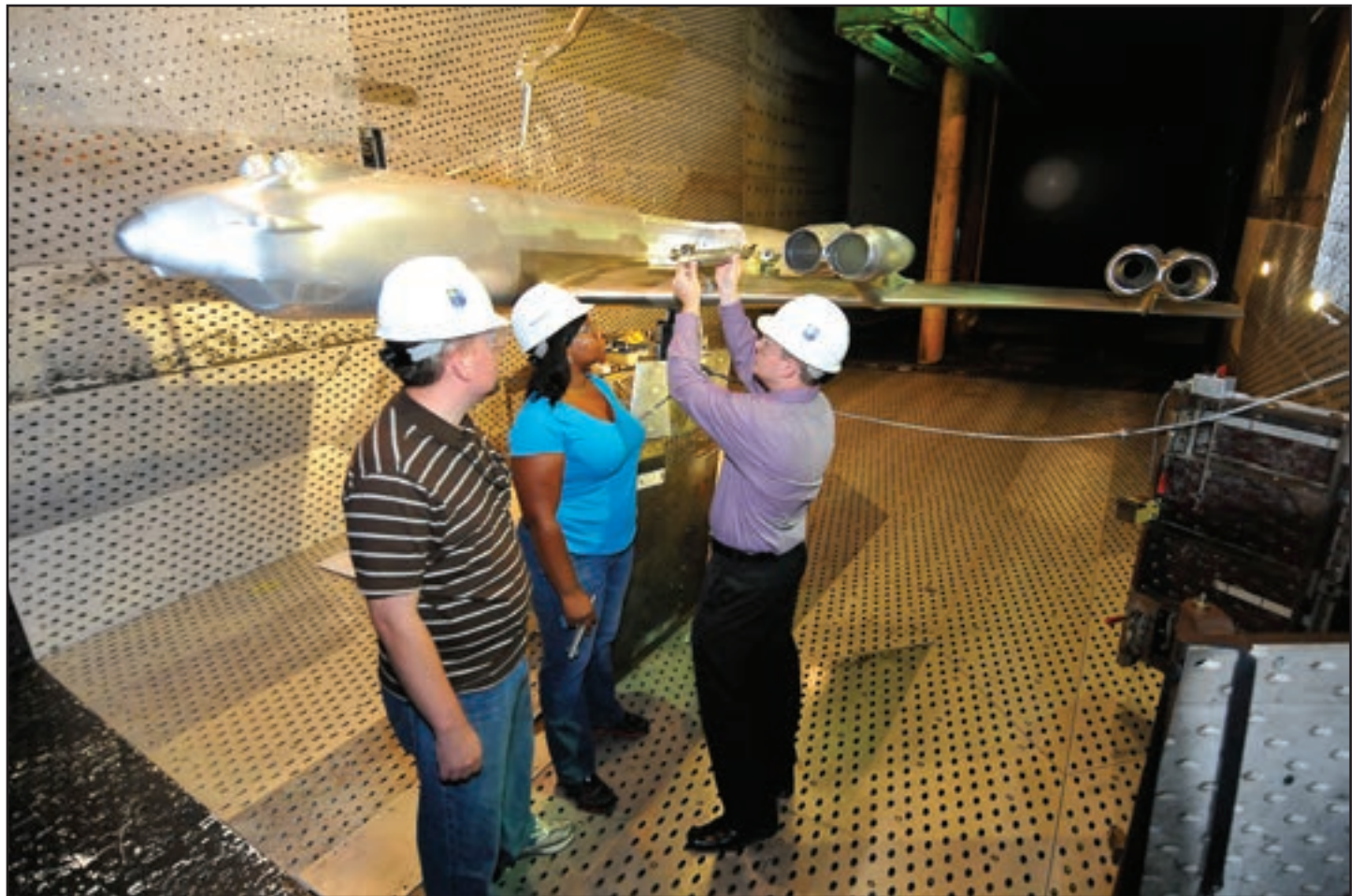
Paul Haas, B-52 Program Office, Tinker AFB, Druana Sanders, Booz-Allen & Hamilton Inc., and Don Arrowood, B-52 Program Office, Tinker AFB, examine the B-52H model's stores in AEDC's 16T between store separation test runs. (Photo by Rick Goodfriend)
