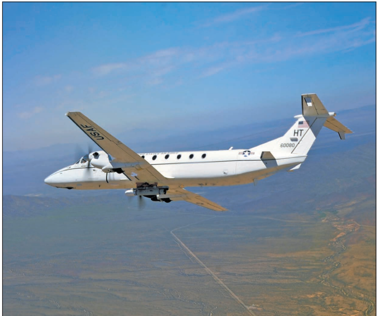
A highly modified Air Force C-12J with an inert Laser Maverick on the belly of its fuselage flies after a testing mission. The Laser Maverick is an air-to-ground missile that can seek out laser-designated targets. The 586th Flight Test Squadron at Holloman Air Force Base, New Mexico, has tested external stores on the modified C-12J, which is normally a "people mover." (U.S. Air Force photo/Airman 1st Class Joshua Turner)
