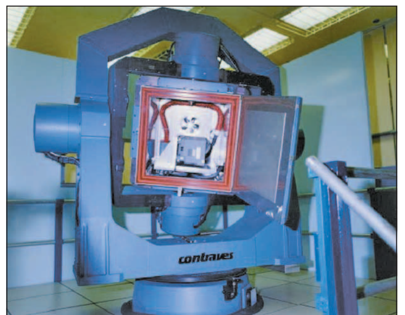
Pictured is the Contraves Model 53Y, 3-axis table centrifuge at Holloman Air Force Base. It is capable of 720 degrees per second rotation, with an environmental chamber and can accommodate a test item weighing 100 pounds. (Holloman AFB photo)
