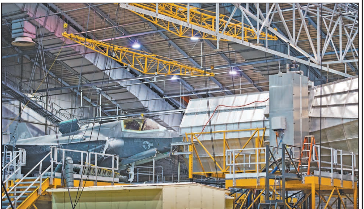
An F-35 endures freezing temperatures in the AEDC McKinley Climatic Laboratory at Eglin Air Force Base, Florida, Jan. 27, 2015. The joint strike fighter underwent four months of climate testing in the lab to certify the fleet to deploy to any corner of the world. (U.S. Air Force photo/Samuel King Jr.)
