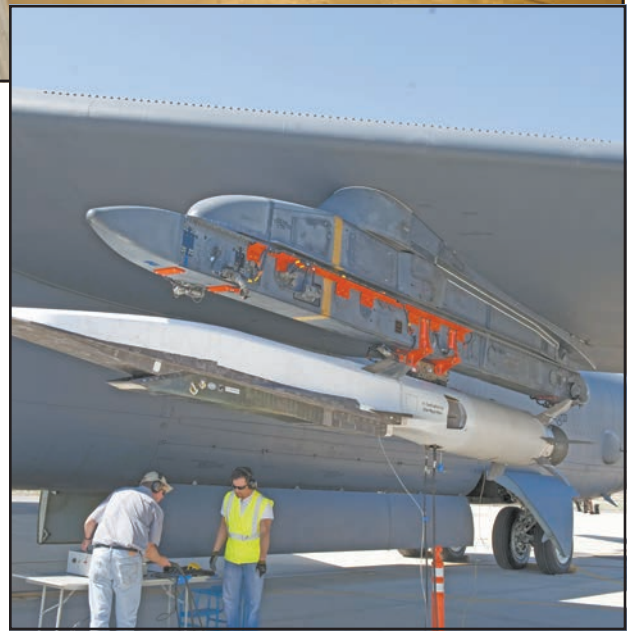
Ground crew members of the Hypersonic Combined Test Force make the final checks to the X-51A Waverider scramjet, which is affixed to an Edwards Air Force Base B-52H Stratofortress before being flown over the Pacific Ocean and launched June 13, 2011. The Hypersonic CTF is a unit of AEDC. (Photo by Bob Ferguson/Boeing)
