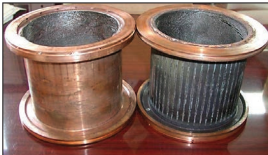
Evaluation of Arc Heater Anode and Cathode Coatings on Wear
