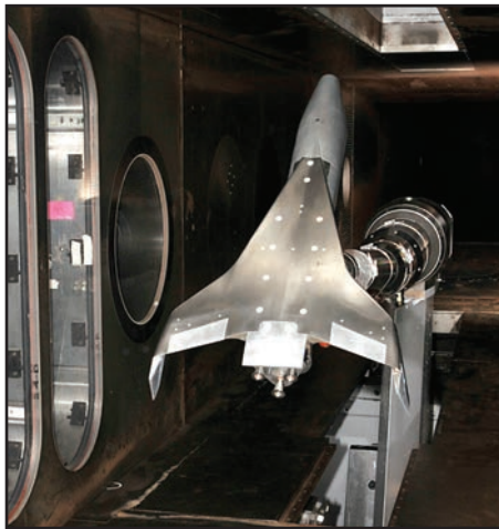
Fully-Reusable Access to Space Technology Proof-of-Concept Launch Vehicle in Tunnel A
