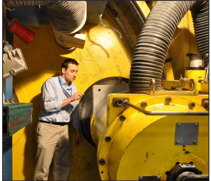
Tire in advanced development of missionized aircraft tire wear testing for the F-35 Lightning II program
