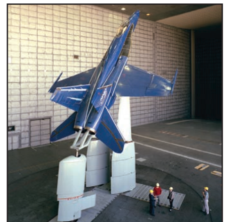
Full-Scale F/A-18 Hornet at High Angle-of-Attack
