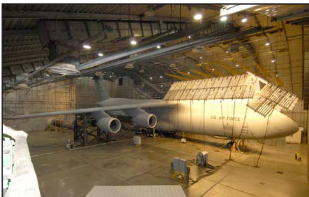
C-5M Super Galaxy extreme heat and ultraviolet exposure in the McKinley Climatic Laboratory
