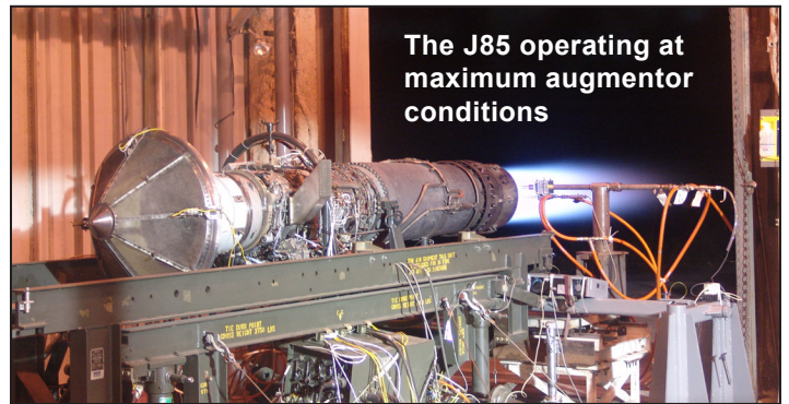
Flow field probing hardware positioned in the engine exhaust
