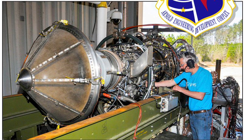
AEDC's upgraded J85 Augmentor Rig coupled to GE's developmental augmentor assembly.
