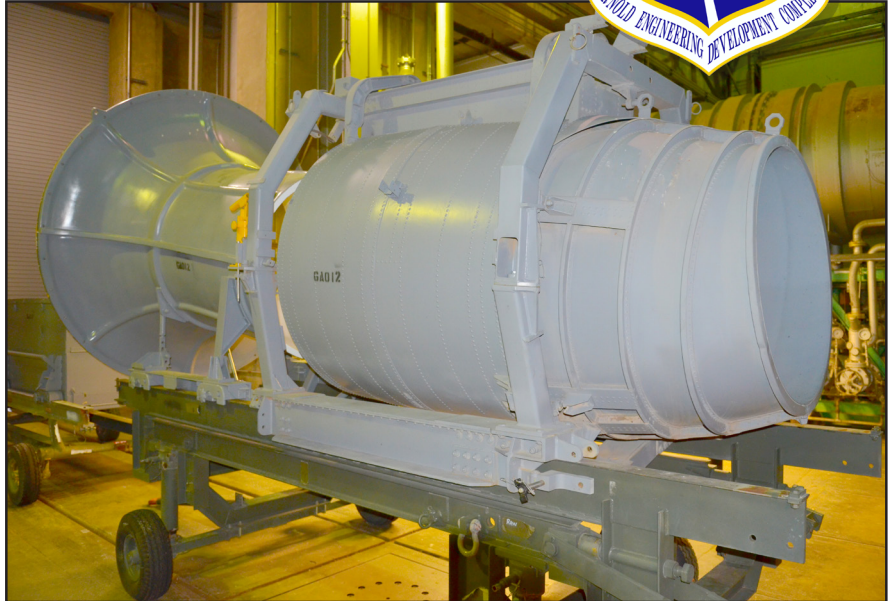
Shown is the adapter portion of the kit where the engine is mounted.
