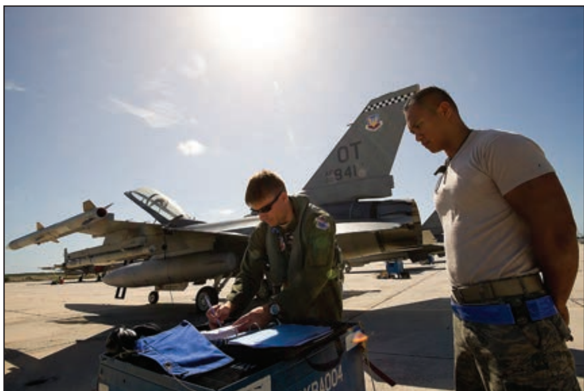
Above, Senior Airman Horacio Maysonet from the 51st Combat Communications Squadron at Robins Air Force Base, Ga., performs set up and testing on radio frequency modules during the Vigilant Shield 12 exercise on Naval Air Station Key West, Fla., Nov. 5. The RFM consolidates radar feeds extending long distances into one air picture allowing higher headquarters to access and engage incoming threats. Below, Staff Sgt. Jam Baro, a crew chief from the 46th Aircraft Maintenance Squadron at Eglin AFB,, and Maj. James Geoppinger review all paperwork before a mission during the Vigilant Shield 12 exercise on Naval Air Station Key West, Fla., Nov. 6. (U.S. Air Force photos/Tech. Sgt. Dennis J. Henry Jr.)
