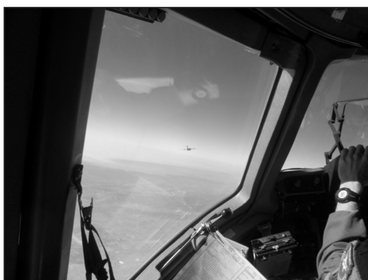
The view from a C-17 cockpit while trailing behind another C-17 during the first tests of "vortex surfing" at Edwards Air Force Base, Calif., Oct. 2, 2012. Early indications from the tests promise a reduction of fuel consumption by up to ten percent. (Courtesy photo)
