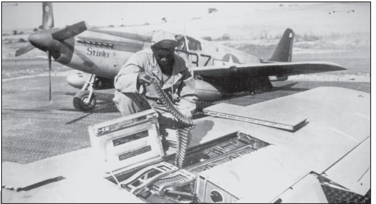
An armorer of the 15th U.S. Air Force checks ammunition belts of the .50 caliber machine guns in the wings of a P-51 Mustang fighter plane before it leaves an Italian base for a mission against German military targets. The 15th Air Force was organized for long range assault missions and its fighters and bombers range over enemy targets in occupied and satellite nations as well as Germany itself. Ca. September 1944. (National Archives photo no. 208-MO-18H-32984)
