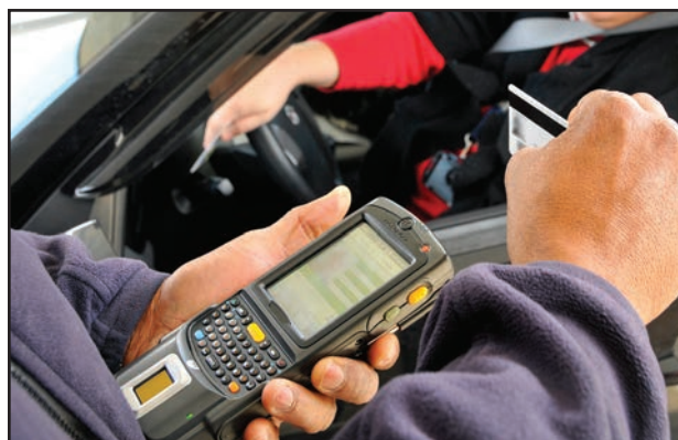
Officer Jim Taylor operates the new Defense Biometric Identification System (DBIDS) as ATA employee MaryBeth Barlow enters the AEDC main gate. The DBIDS scans an individual's Common Access Card (CAC) or similar DOD credentials when they enter the base security gates. (Photo by Jacqueline Cowan)
