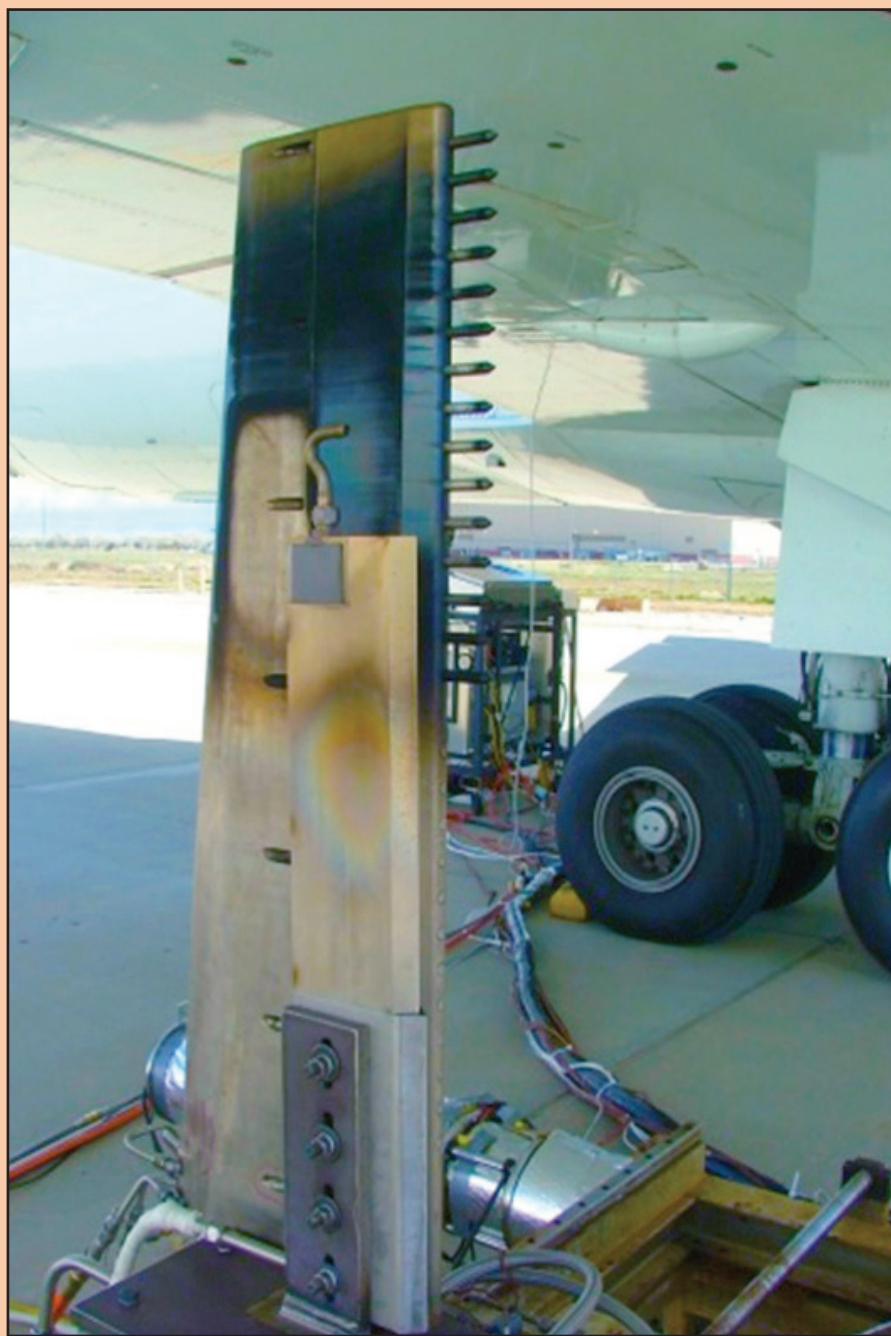
The NASA Alternative Aviation Fuel Experiment-II (AAFEXII) AEDC team tested NASA's DC-8 aircraft CFM-56 engines for emissions using a rake positioned behind the right inboard engine. (NASA photo)
