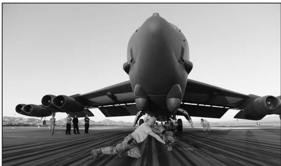
Senior Airman John Myer pushes a tow bar under the tire of a B-52H Stratofortress during a Red Flag exercise at Nellis Air Force Base, Nev. The B-52 shredded a tire upon landing after a four-hour mission. Myer is a B-52 aircraft maintainer assigned to the 2nd Aircraft Maintenance Squadron at Barksdale AFB, La. (U.S. Air Force photo/Staff Sgt. Vernon Young Jr.)
