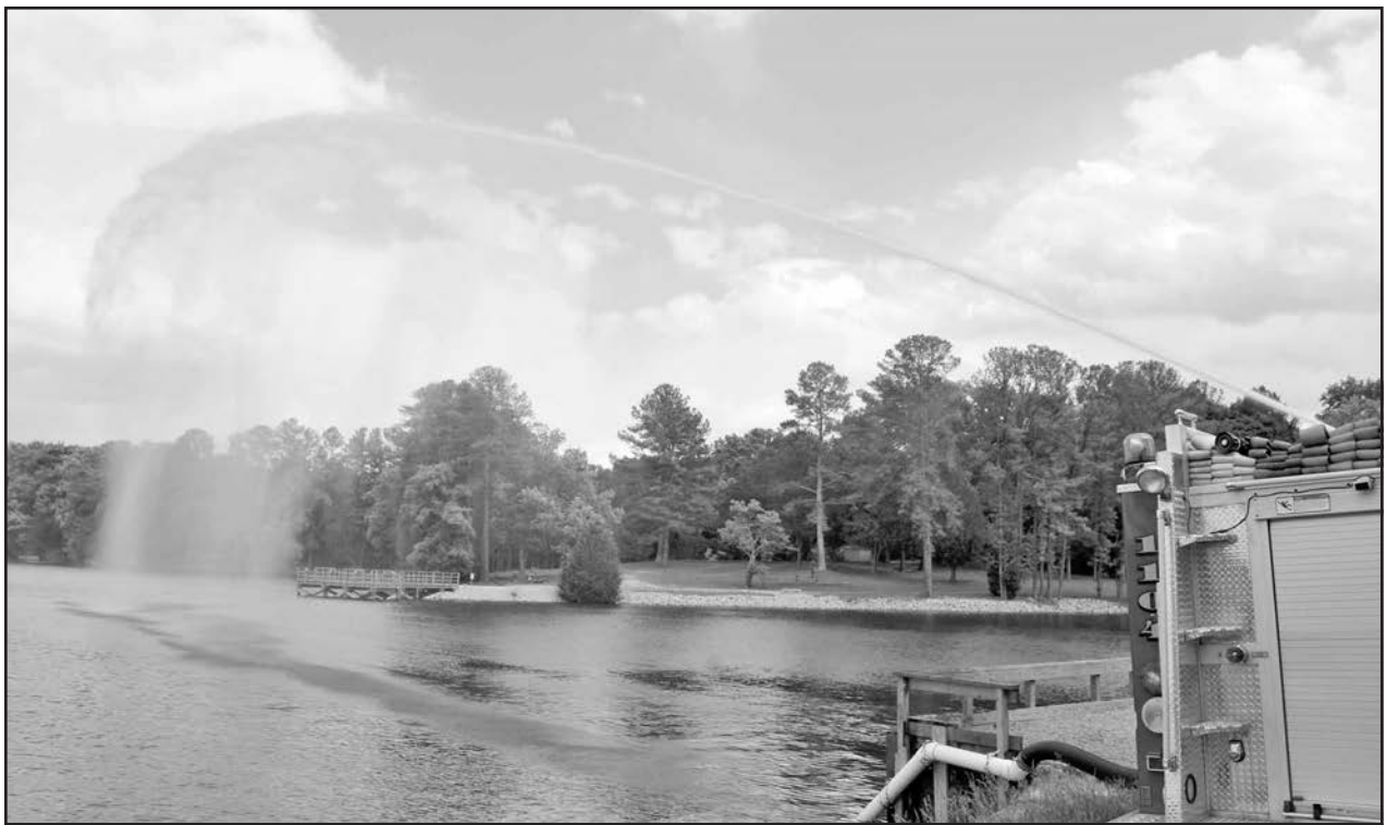
Members of the Capitol Hill and Arnold Air Force Base fire departments work together to perform a first draft of the dry hydrant installed at Morris Ferry Dock. Pictured in the first photo are Capitol Hill fire personnel hooking the fire truck up to the dry hydrant. As seen in the second photo, the fire hose successfully sprays water from the lake. Pictured in the last photo are AEDC fire personnel Odell Crutchfield (left) and Billy King (right) assisting in detaching equipment from the truck. (Photos by Jacqueline Cowan)
