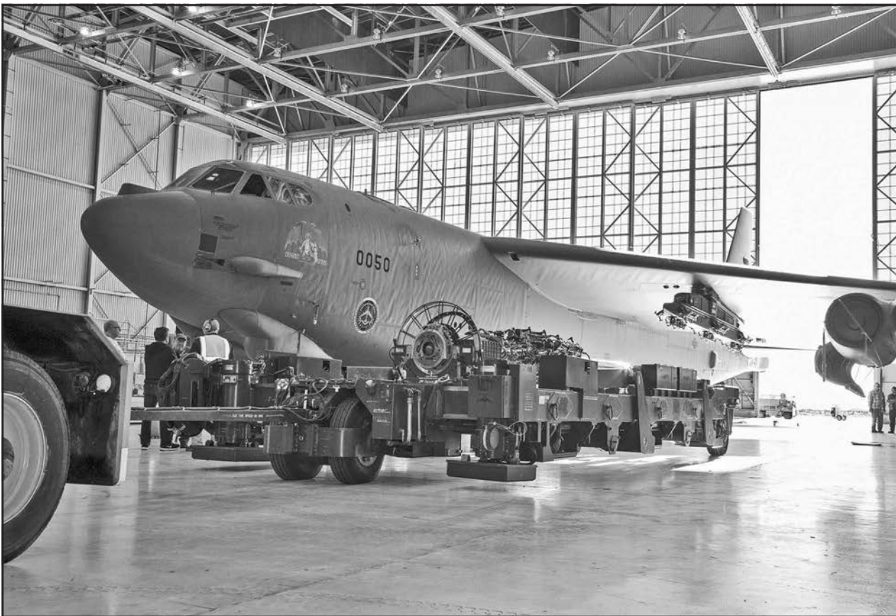
Team members from the 419th Flight Test Squadron, the Global Power Bomber Combined Test Force and Boeing installed a Conventional Rotary Launcher (CRL) December 2014, on a B-52H Stratofortress from Edwards Air Force Base, Calif. The upgrade modifies the internal weapons bay of the B-52H by integrating a CRL that has the capability of carrying Military Standard 1760 “smart weapons.” (U.S. Air Force photo/Bobbi Zapka)
