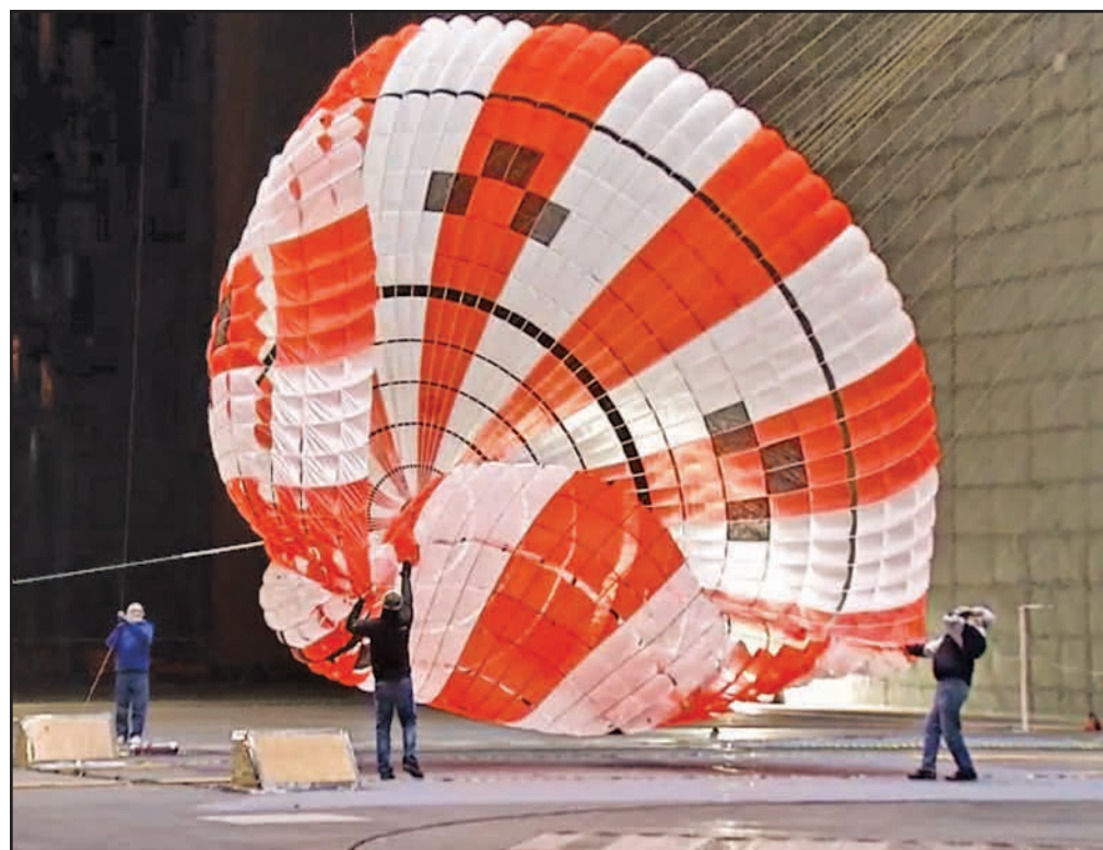
AEDC engineers were part of a test team that performed wind tunnel testing on the parachutes for NASA Orion spacecraft in January. The test team also consisted of NASA, Airborne Systems, Jacobs Engineering and NFAC personnel. Pictured here is a parachute being tested in a NFAC wind tunnel. (AEDC photo)
