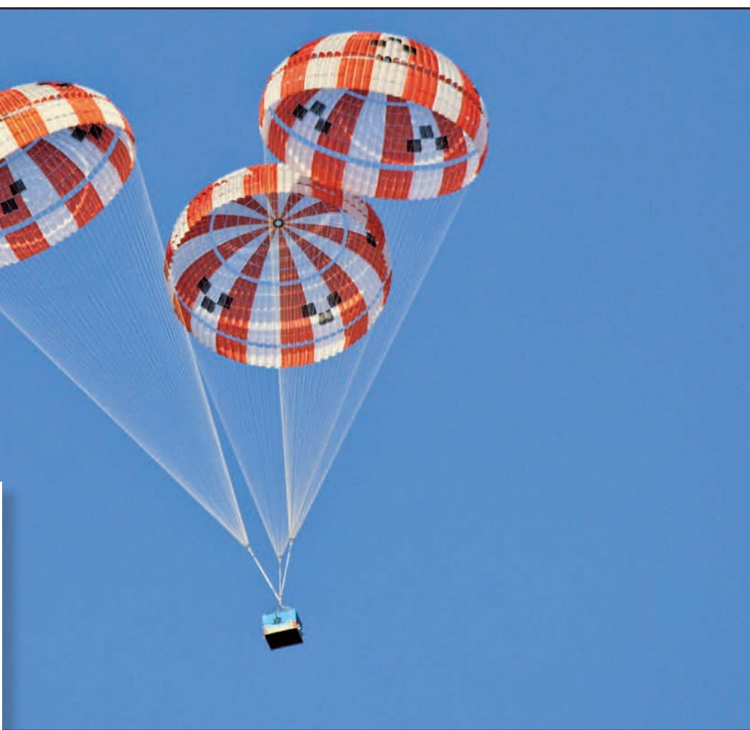
On Feb. 2 in Eloy, Ariz., engineers performed air drop testing on sub-scale parachutes for the NASA Orion spacecraft. The test is meant to determine which parachute configuration will ensure the Orion lands safely after missions. (Photo credit: NASA)
