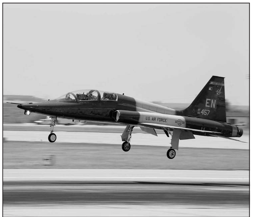
Pilots practice touch-and-go maneuvers in a T-38 Talon during training at Sheppard Air Force Base, Texas. The Talon is a two-seat, twin-engine supersonic jet trainer used to train pilots in the international Euro-NATO Joint Pilot Training Program. The pilots are assigned to the 80th Flying Training Wing. (U.S. Air Force photo/Danny Webb)
