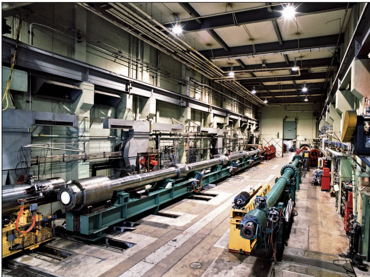
A technology project is taking place in Range G at AEDC to prepare for advanced hypersonic testing. Pictured here is the inside of the Range G impact and ballistic launch facility. (AEDC file photo)
