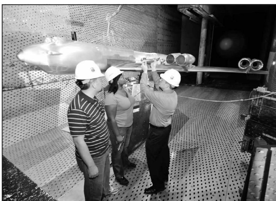
Pictured left to right is Paul Haas, B-52 Program Office, Tinker Air Force Base, Druana Sanders, Booz-Allen & Hamilton, Inc., and Don Arrowood, B-52 Program Office, Tinker AFB, as they examine the B-52H model stores in the AEDC 16-foot Transonic wind tunnel between store separation test runs. The tests, conducted in 2011, contributed to increased capability for the B-52. (U.S. Air Force photo/Rick Goodfriend)
