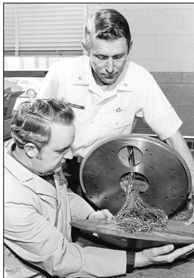
Extensive instrumentation required on the NASA Viking model is shown here before a test at AEDC in 1973 before final assembly. There were 68 sensors to record localized heat buildup around protrusions on the face of the Mars entry vehicle, while 13 heat and five pressure sensors were installed on the base cover. Then Maj. Dale Holasek of the AEDC Directorate of Test watches the assembly by Ray Moore, a test facility craftsman. (AEDC photo)
