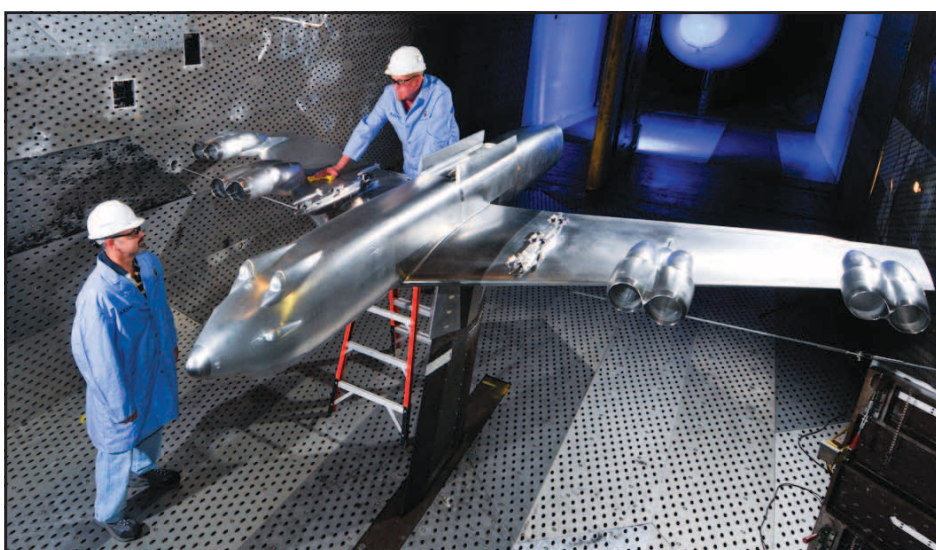
AEDC set a record for the largest aircraft model used in conducting store separation tests of the aircraft with a 10-percent scale model of the B-52 Stratofortress. The testing was requested by the B-52 Program Office of the Air Force’s Global Strike Command to validate separation of multiple weapons that previously had not been released from the B-52 weapons bay. Results from the test data and subsequent analysis gave the program office confidence to increase the B-52’s guided-weapon capacity. Pictured from left is J.T. Thompson, captive trajectory system project engineer, with Gary Cunningham, lead outside machinist, in the AEDC Propulsion Wind Tunnel 16-foot wind tunnel between store separation test runs in 2011. (U.S. Air Force photo/Rick Goodfriend)
