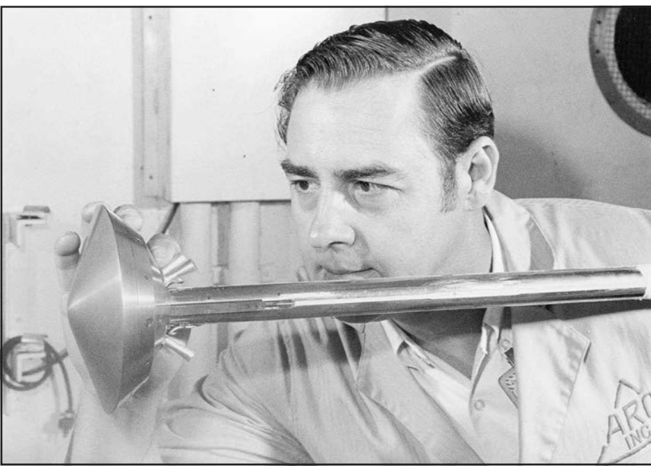
The NASA Viking Mars Probe is set up here in 1971 for a free flight test at the AEDC von Kármán Gas Dynamics Facility by drilling a hole through the diameter of the two-inch models and suspending them on a wire. A system of pulleys and weights held the wire taut while the desired conditions were established inside the wind tunnel. Sudden force applied to the ends of the wire caused it to break within the model, leaving the model unsupported for a brief interval. This permitted engineers to examine the airflow, not only around the model, but also in its wake. Airflow is from left to right. Observing the test arrangement is then F.L. Badman, a test engineer. (AEDC photo)
