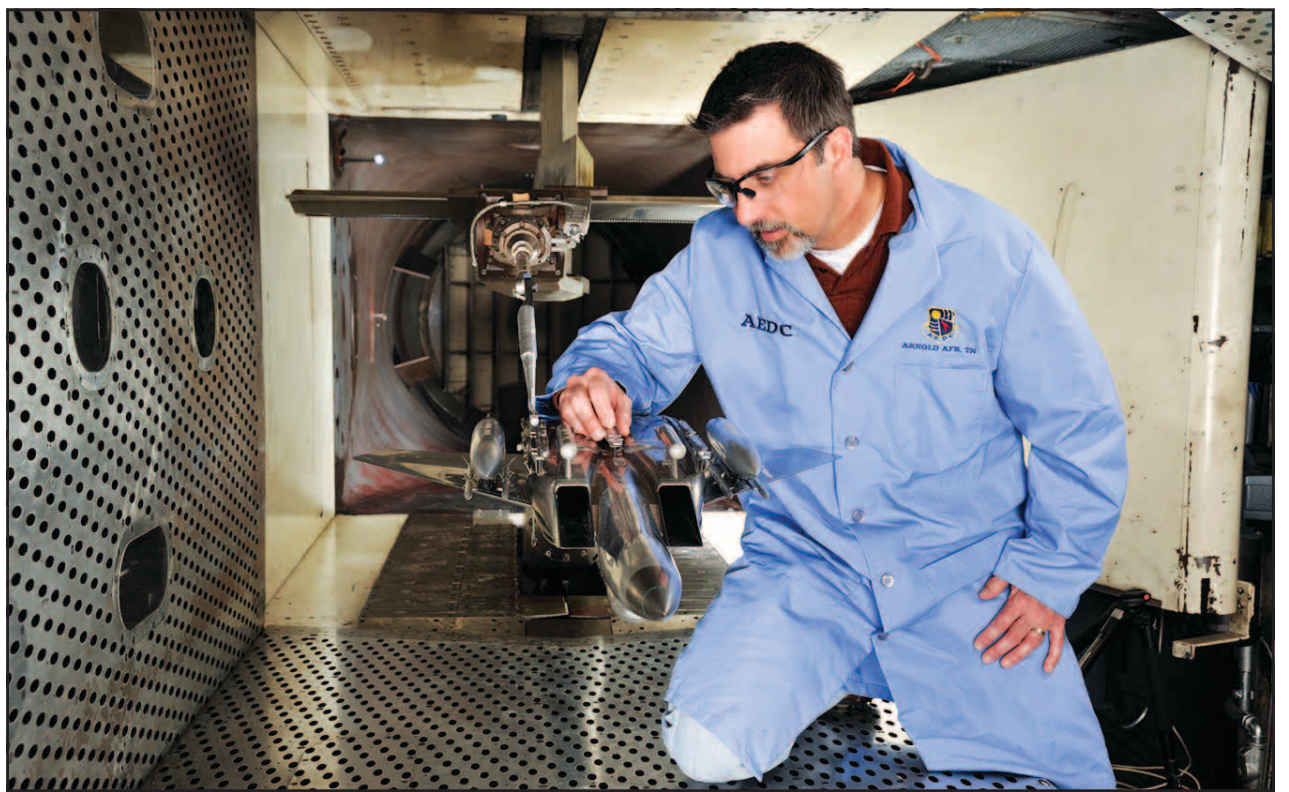
AEDC Team Member David Anderson inspects 1/20-scale models of the F-15E Strike Eagle aircraft and sting-mounted Small Diameter Bomb II, during a break in ongoing store separation tests for new weapons development phase trials in the 4T wind tunnel of the Propulsion Wind Tunnel facility. (U.S. Air Force photo/Rick Goodfriend)
