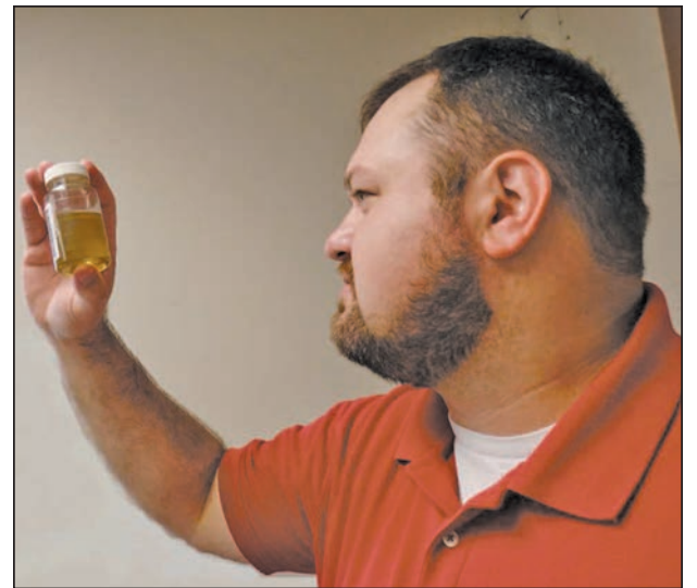
Casey Schewe, Oil Analysis/Processing Program lead, examines a sample of oil taken from a hydraulic unit. Preventative maintenance efforts like this are part of the Asset Health Assurance program at AEDC, which is a long-term reliability and maintenance program for the Test Operations and Sustainment contract. (AEDC photo)
